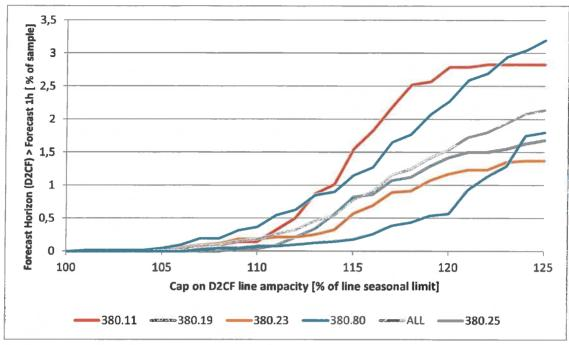
This graph shows the occurrences where the Forecast Horizon is higher than Forecast 1h (ordinate axis). We observe that the Forecasts Horizon values capped at 105 % of the seasonal limit presents a robust confidence margin (~100%).
